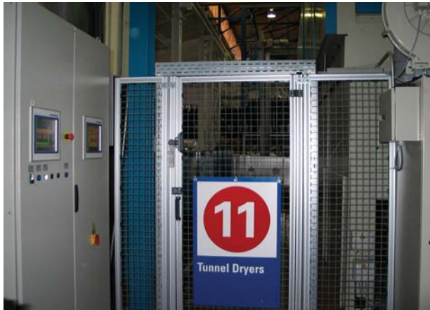
The tunnel washer, conveyors and other heavy machinery is secured with fencing, gates and automatic shut-off sensors. Various departments are identified by numbered signs.
