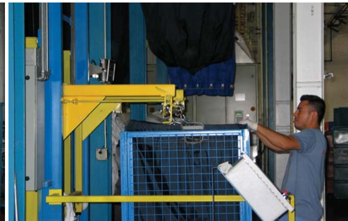
An employee checks a sling that's attached to an automated lift system.
