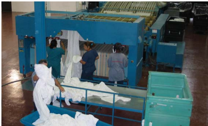
A view from a raised platform shows employees feeding textiles into a spreader/feeder
